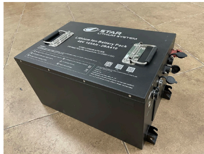
2BA410 105Ah Lithium Battery
